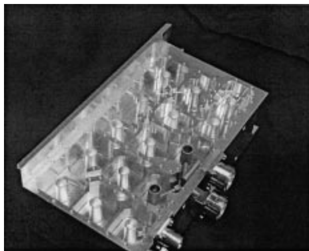
Fig. 14. Coaxial resonator realization of a cellular radio base-station filter.
